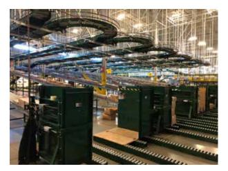
the facility with an inbound automated storage and retrieval system with nine aisles, as well as an automated bagging system for completed orders that is capable of bagging 900-plus packages an hour. The entire fulfillment center is designed to minimize the number of times product is touched between receiving and shipping.
