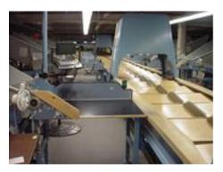
One facility: Freeport Maine – VAS system design (existing operation re-design), sortation machine (Crisplant – VAS optimized sort control), tote management (VAS controls), workstations, conveyance controls. Optimized carton sortation.
